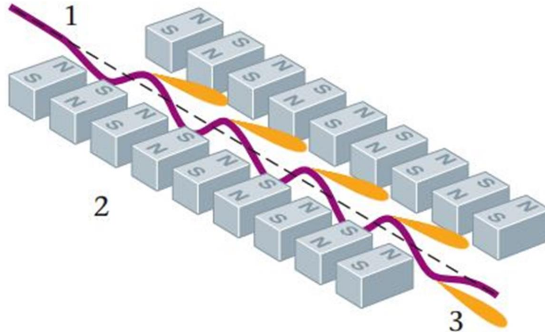
▲ FIGURE 22-18 In a synchrotron undulator, a beam of high-speed electrons (1) passes between the poles of a series of alternating magnets (2). This undulates (or wiggles) the beam, causing the electrons to emit X-rays (3).
